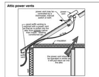
Attic fans are generally mounted on the outside of the roof structure or in a gable end. They are usually activated by a thermostat. As the temperature increases, the fan will go on automatically.
